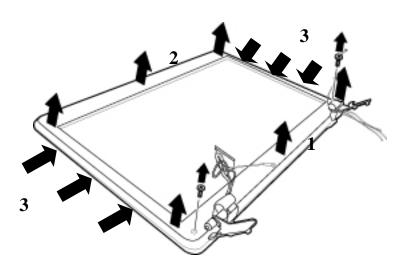
Figure 4-45 Removing the bezel
